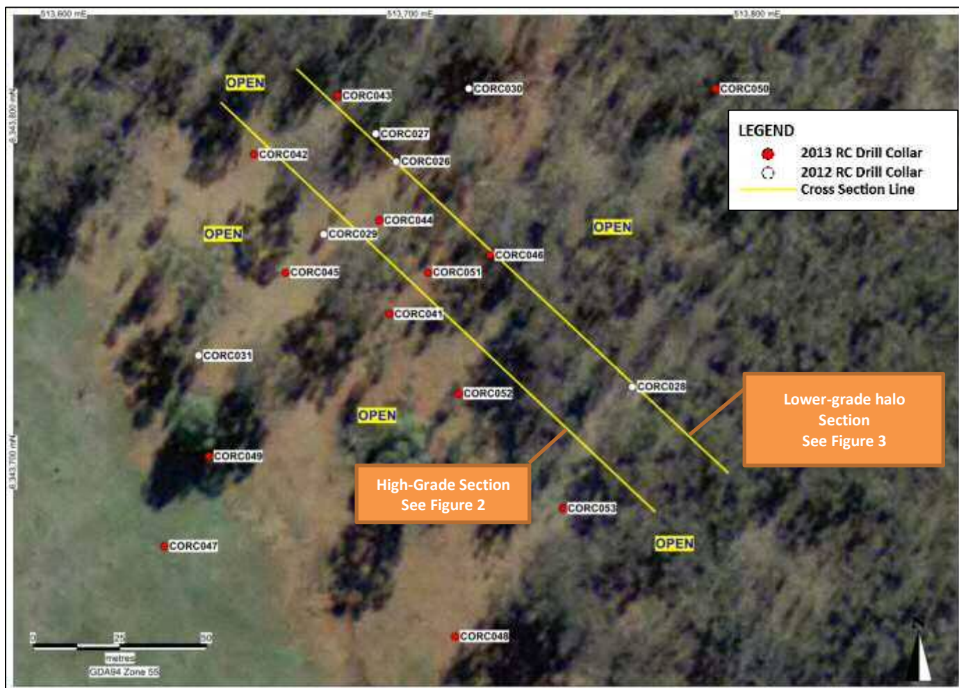
Figure 1 - Plan view of RC drill program over the Meritilga Prospect lode zone. Included are drill collars from the 2012 RC program, some of which are depicted on cross – sections in Figures 2 & 3.
