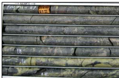
NQ drill core from hole FVD001 between 156m and 162.5m. Note the intense epidote alteration (green) near the bottom of the photo.
